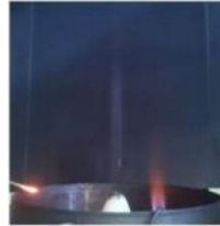
Sydney lean H 2 /air jet in hot coflow
