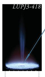
Pilot flame d = 61 mm Phi = 0.9 u = 0.3 m/s Fuel/air Jet d = 1.5 mm Phi = 0.4 66 m/s < u < 418 m/s
