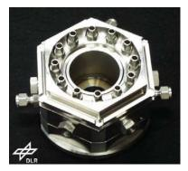
Fig.1: Photo of a gas turbine combustor based on jetstabilized flames
