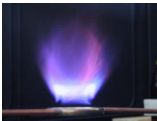
Figure 2 shows one example of the flame, seen from side, the flame is clearly detached from the burner.
